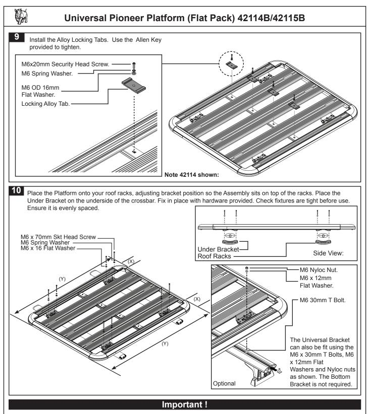
Do not connect eyebolts in outer extrusion, connect only to planks. 'T' Bolt connection must be used.
